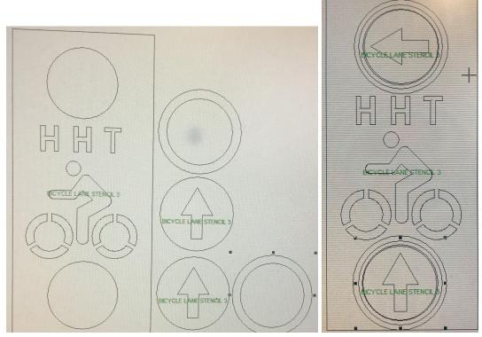
This will have rotatable arrows for use in any direction Printed stencil approx: 48" x 20"
